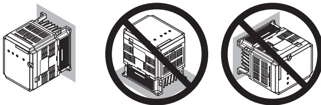
Figure 8 Correct Installation Orientation (Braking Unit)
